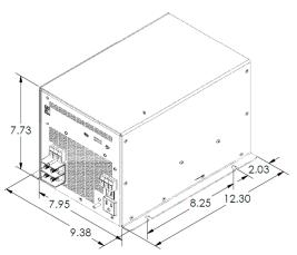
The heavy-duty toroidal power transformer inside the inverter weighs 30+ pounds. Unless the unit is mounted horizontally, it could break free from its single mounting bolt under severe vibration.
