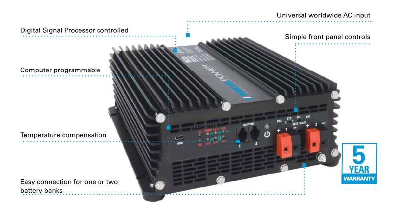
The IBC series chargers are fully Digital Signal Processor controlled and feature Universal Input Voltage from 85 to 265 VAC at 50 or 60 Hz with Active Power Factor Correction for the most efficient use of AC power.
