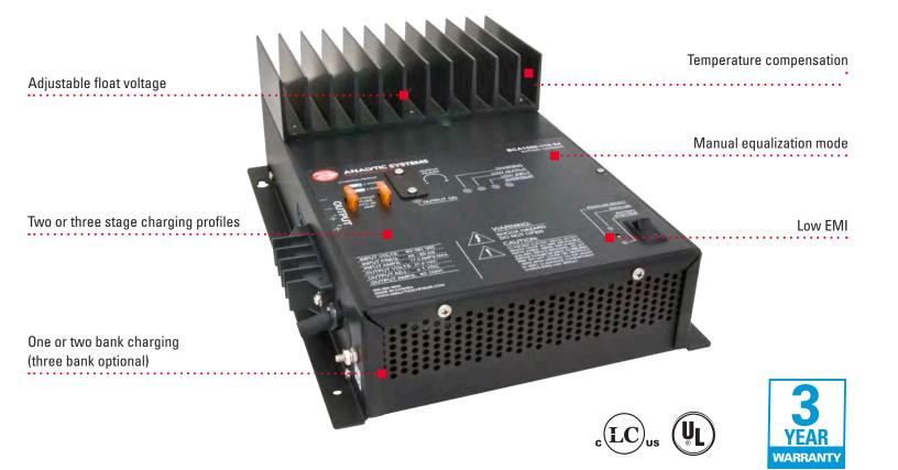
The BCA1000 provides up to 1000 watts of precision charging power to up to two banks of batteries at 12, 24, 32, 36, 48 or 72(rail) volts DC from a 110 or 220 volts AC power source. The output voltage is easily adjusted 1.0 volts above or below the standard output voltage for standard or deep cycle lead-acid, VRLA or Gel cell type battery.
