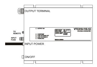
Allow at least 1 inch of clearance all around the case for cooling. The best mounting configuration is to mount the unit on a vertical surface oriented as shown. Use #10 screws of the appropriate type for the mounting surface to securely mount the unit.
